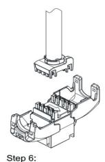
Put the cap on the IDC tower. The arrows on the jack and the cap should face the same direction. Put the cap into position.
