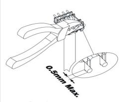
Step 4: Cut the excess wires off. The tips of the wires should protrude no more than 0.5mm.
