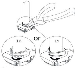
Step 5: Wrap the grounding wire,braid around the cap as shown picture (Leave at least 7mm for grounding)
