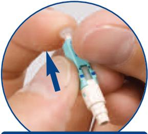
2. Slide Activator Tab to the Open Position
